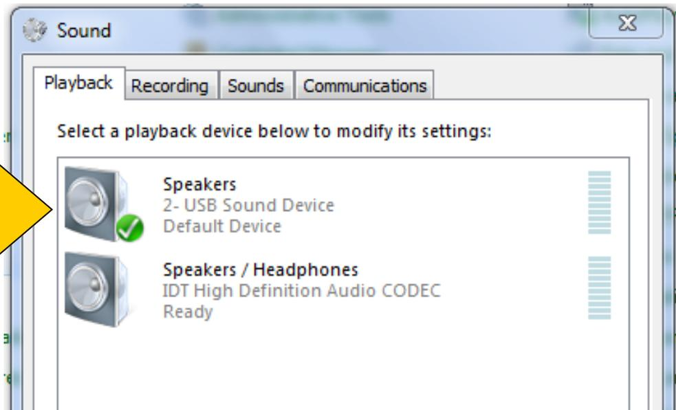
Once this is complete, the speaker will automatically configure and take over when your tablet is in the dock. If you remove the tablet, the computer’s internal speaker will take over.
