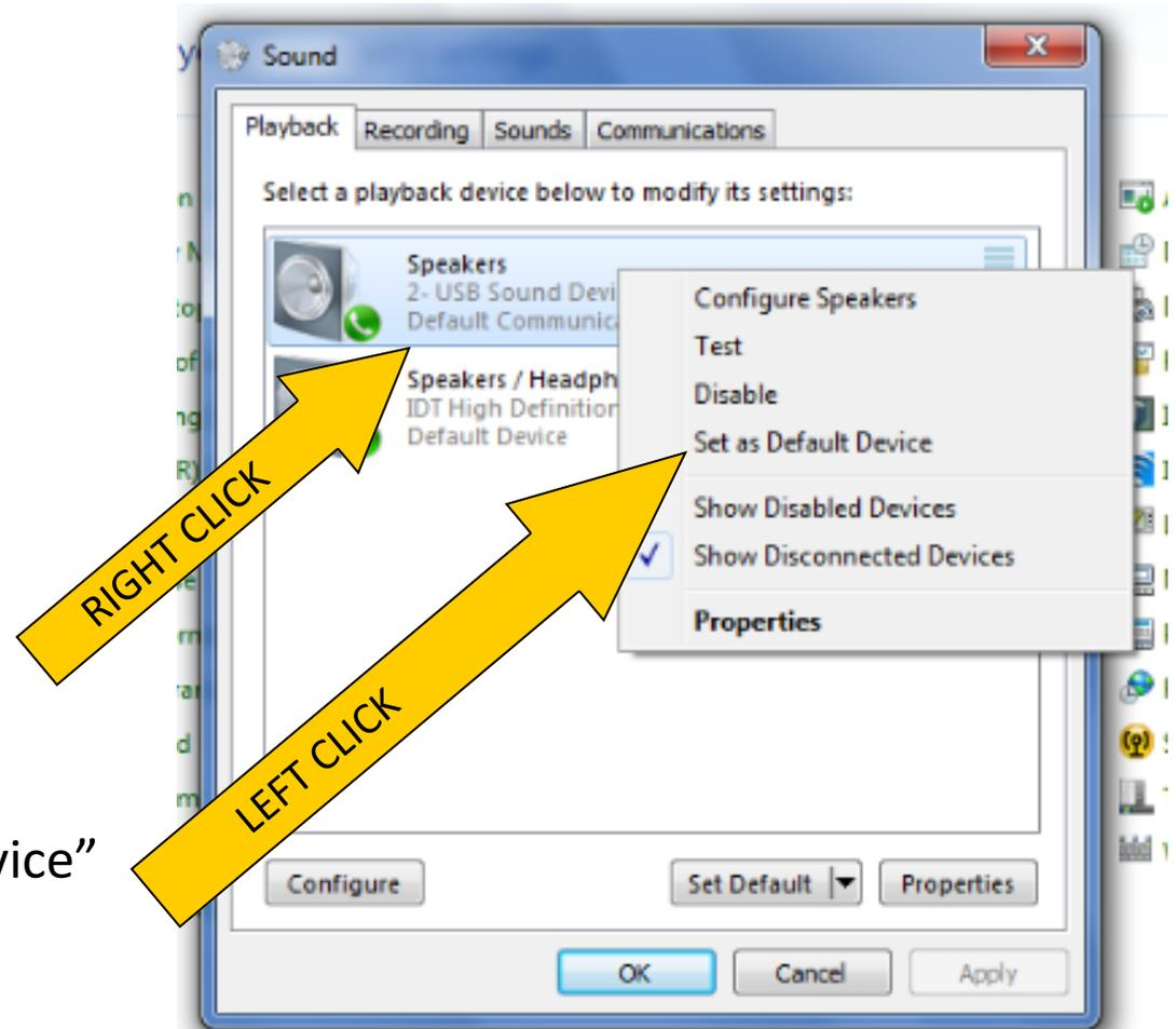
Once completed the USB speaker should have a green checkmark and be listed as “default device”.
