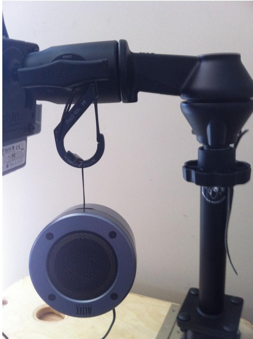
Ensure that the location you choose leaves enough slack in the USB cable to allow any articulation in the tablet that you may want. Once installed connect the USB Cable to a port under the mobile docking station.
