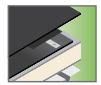
**Battened-Seam Systems** provide exceptional strength and integrity on applications where 7.5' (2.3 m) or 10' (3 m) wide GenFlex EPDM or FRM membrane is used. (IMAGE AT LEFT)
