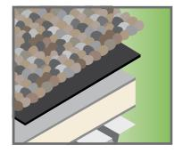
**Ballasted Systems** are perfect for installations where speed and economy are prime considerations, and the substrate is capable of supporting the system's dead load. Slope must not exceed 2" (50.8 mm). Insulation and membrane are loose-laid with the membrane fastened only at the perimeter. Recommended ballast is smooth, water-worn rocks.
