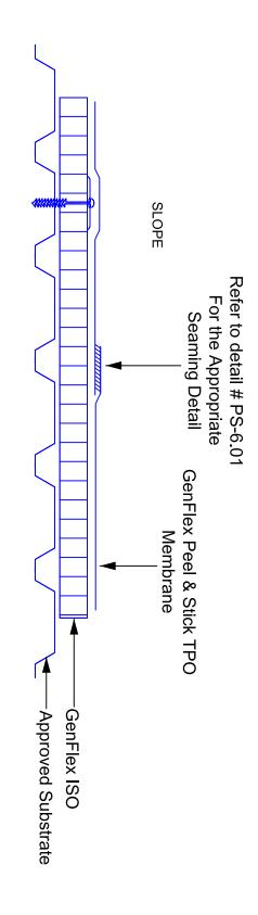
attachment and to reduce fastener movement. Insulation should be installed with board edges resting on the top flutes. Position insulation to enable securement into the top flutes on steel decks to ensure positive
