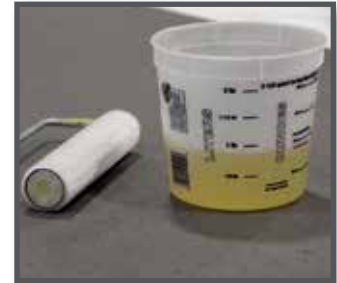
Amount of adhesive needed to cover 4' x 8' at a coverage rate of 150 ft 2 per gallon.
