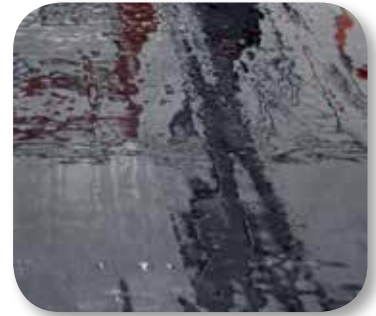
X Heavy Coverage Thick, pooled areas will cause blistering.
