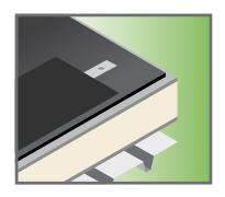
**Mechanically Attached Bar Anchor Systems** provide exceptional strength and integrity on applications with large, open roof areas. These systems include Battened-Seam (IMAGE AT LEFT) and Batten Cover Tape (NOT SHOWN) systems.
