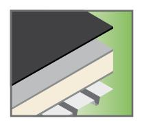
**Self-Adhered Systems** are easy to install, help reduce labor costs and improve worksite air quality. The factory applied pressure-sensitive Secure Bond™ Technology adhesive eliminates field application of bonding adhesives.
